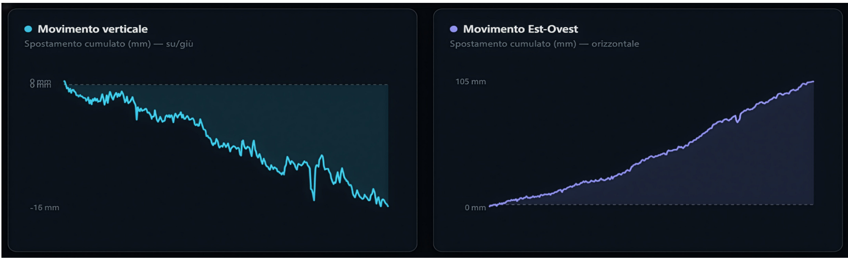
Fig. 2 — EGMS vertical (left) and East-West (right) ground-motion trends for measurement points associated with the Bucchianico school site and used in the ORSS screening analysis.
