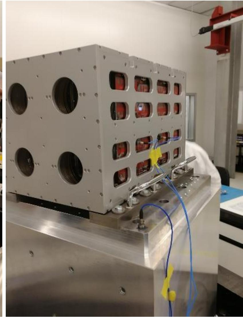
µSADA - Miniaturised Solar Array Drive Assembly for 6U/12U CubeSAT
