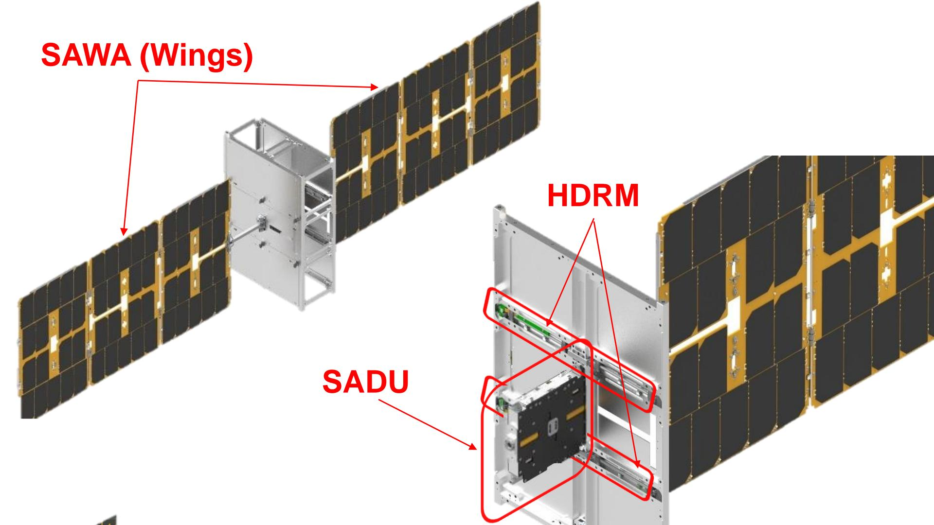
$\mu$ SADA - Miniaturised Solar Array Drive Assembly for 6U/12U CubeSAT
