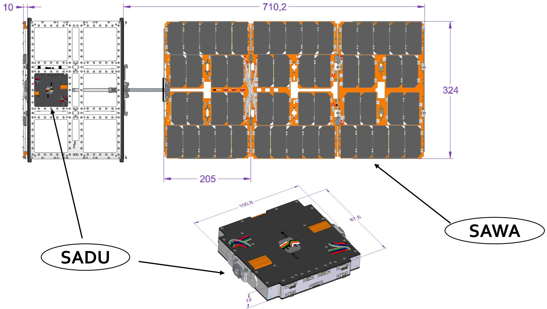
µSADA - Miniaturised Solar Array Drive Assembly for 6U/12U CubeSAT
