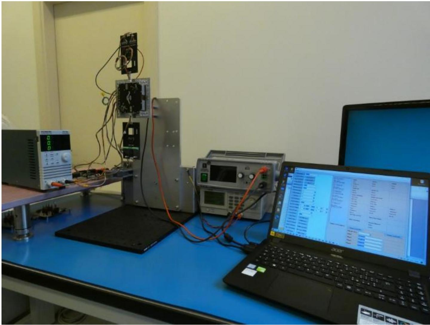
µSADA - Miniaturised Solar Array Drive Assembly for 6U/12U CubeSAT
