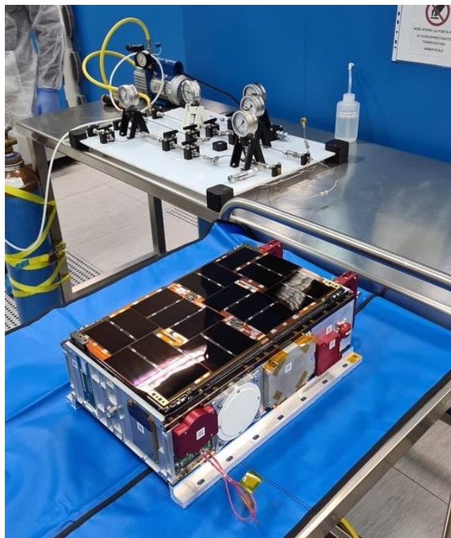
Propulsion System (IANUS) loading with He
