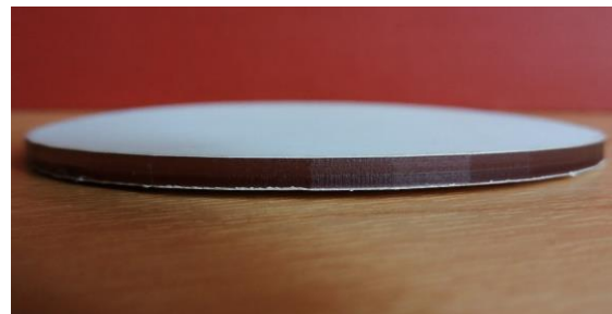
NIKA2 MHWP prototype (~100 GHz - 300 GHz, 200mm Ø, 4mm, 120g)
