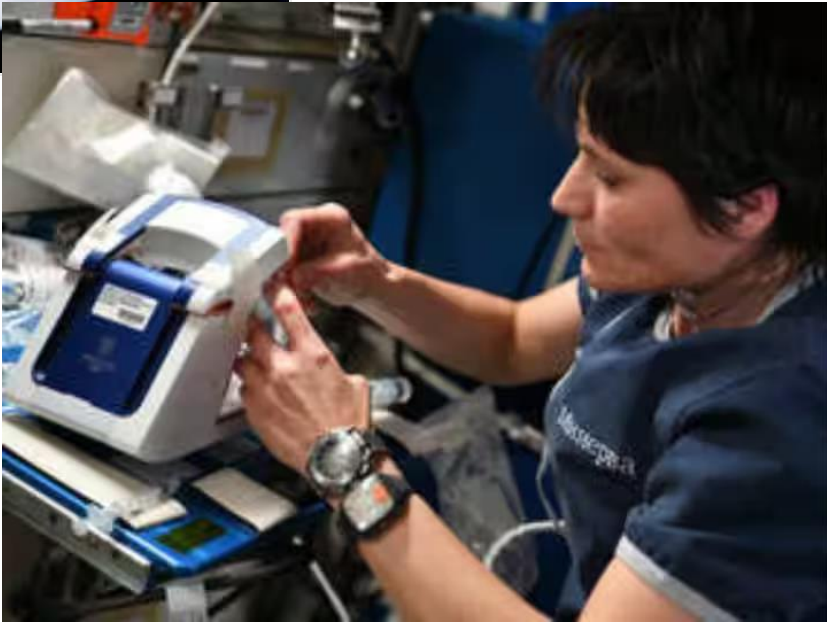
The astronaut Samantha Cristoforetti collects a single biological sample, which could be blood, saliva or urine, on a nanostrip. The strip is inserted into the device. ( Image Source : NASA )
