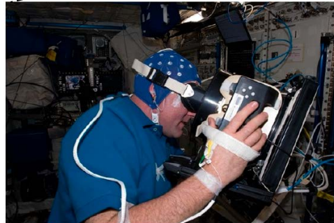
Figure 1. Data collection with an EEG electrode cap onboard the ISS. European Space Agency (ESA) astronaut Andre Kuipers is wearing an EEG electrode cap for the NEUROSPAT investigation. (NASA Image: ISS030E022613).
