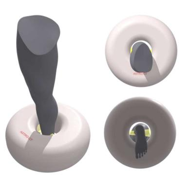
A compact micro-CT system with spectral capabilities (Timepix4 hybrid pixel detectors) for assessing bone density loss in astronauts while onboard the International Space Station.
