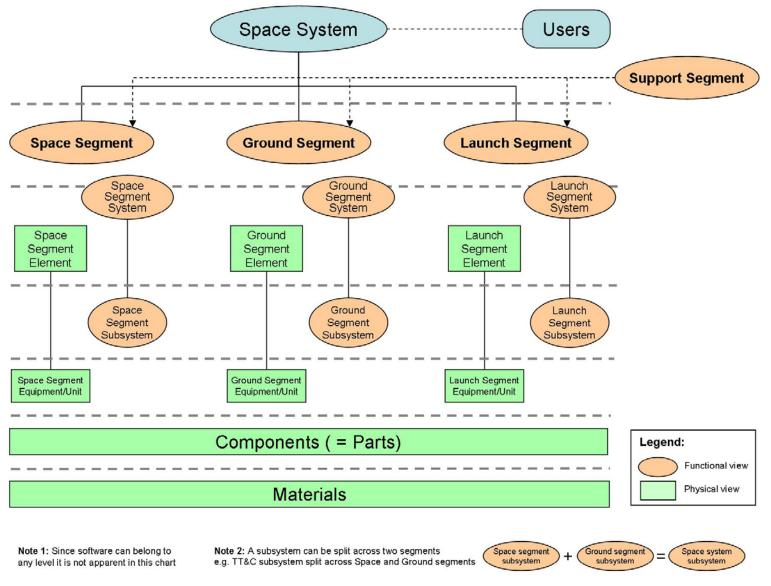
Figure 2-1: Space system breakdown
