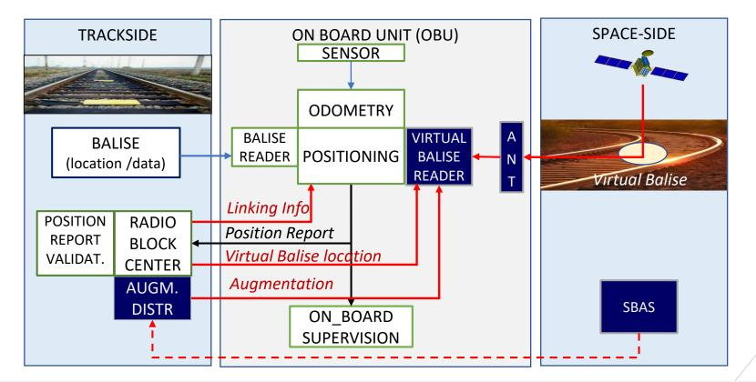
The GNSS Location Determination System generates the same signals produced by a Balise Reader detecting a physical Balise, through the same logical and physical interface, then emulating the Balise reader behavior with respect to the train equipment. In this way the On Board ERTMS/ETCS location determination functions do not need to be changed.
