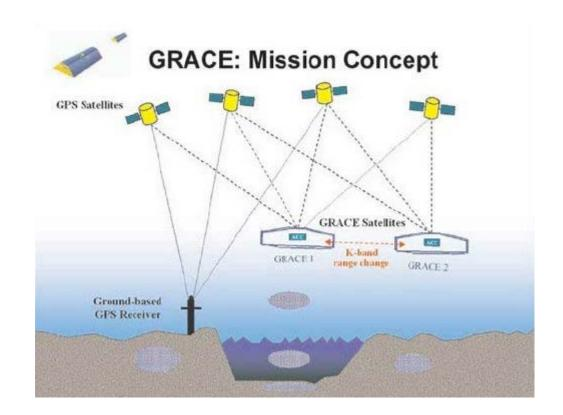
Concept of SST between two LEOs s/c using GNSS was demonstrated with the GRACE mission
