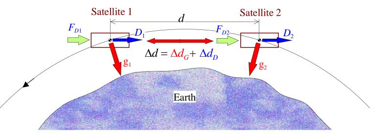
"gravity sensor" consisting of a pair of satellites flying in loose formation; gravity field recovered from measuring (with a laser ranging system) the distance variation ( $\Delta d$ ) induced between the satellites;
