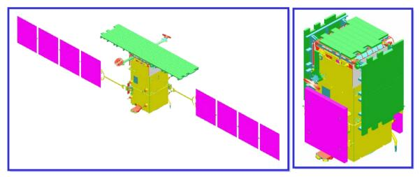
Figure 3 - SAR Satellite (Deployed and Stowed Configurations)
