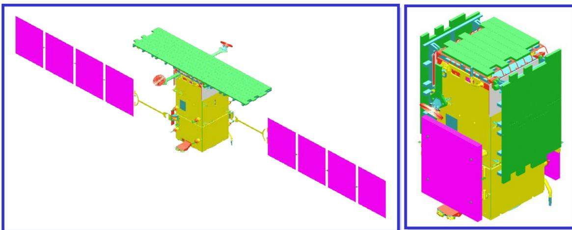
**Figure 3 - SAR Satellite (Deployed and Stowed Configurations)**
