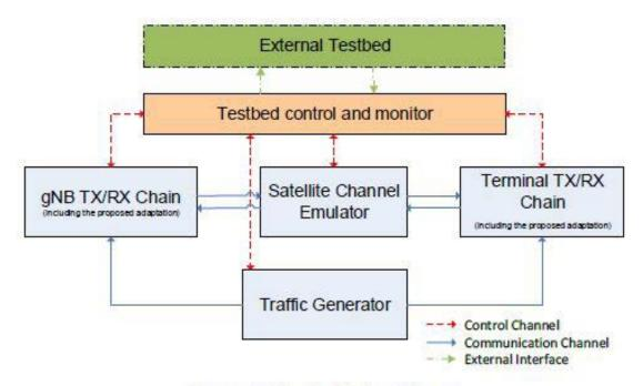
Figure 1: Verification Platform Diagram
