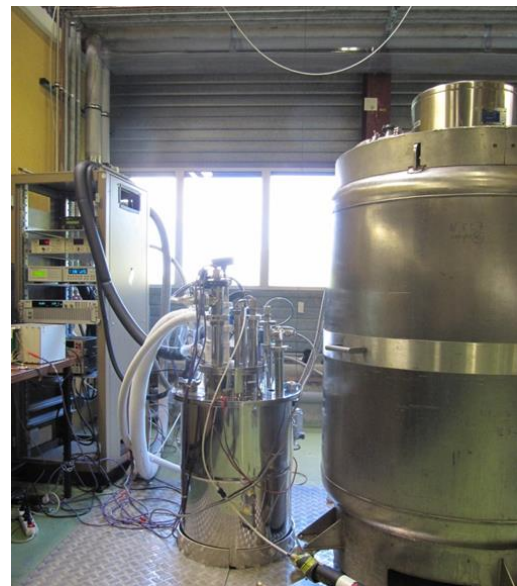
Figure 2: Experimental facility allowing to create a stable superfluid helium bath from 1.4 K to 2.15 K with a constant temperature regulated to the millikelvin. At the center the cryostat and on the left, the data acquisition system and cryostat monitoring.
