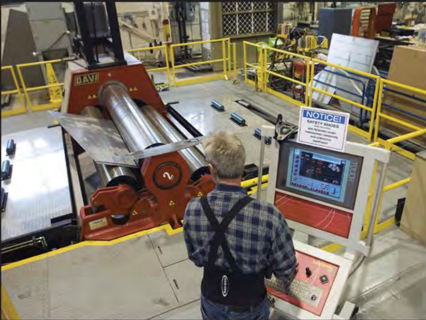
Side Panel Fabrication A side panel is bent the proper shape to be attached to the side of the simulated crew module.
