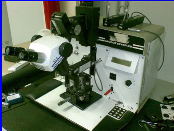
Bond Pull and Die Shear Test
